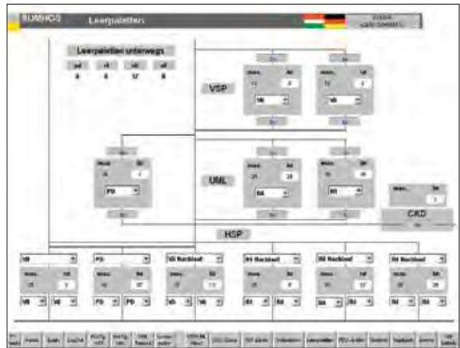
in blocks and then prepared for further transport. Additionally, the conveyor system has a reception station before the main storage locations. This way engines can, on demand, be pulled out of the circulating conveyor and sent directly to the desired dispatch location through a highway. This happens, for example, with custom made engines.
