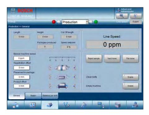
The production display informs the user at Bosch Packaging Systems about all relevant parameters. The upper screen section shows information on the product dimensions (left) as well as machine speed (right). The user can use each input field (center of screen, left) to make offset corrections to the product or foil positioning.
