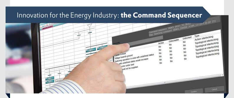
The Command Sequencer simplifies project configuration and setting command sequences massively. The operator can, intuitively and without programming knowledge, compile sequences of commands, test these and apply them. The same also applies for changes in the command sequences. Project configuration is carried out in a graphic editor in Runtime, either by means of selection and compilation of the individual steps, or by means of teaching. With teaching, the system
