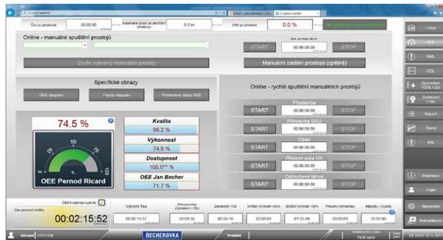
An up-to-date OEE overview is always available on the panel, which is access-protected via a RFID login, and online via web clients – without manual data collection.
