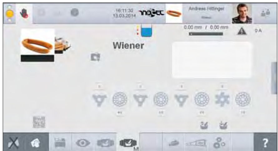
The recipes can be selected using pictures (top left) or a barcode scan.
