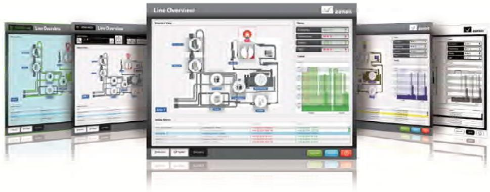
Figure 7: Developed by designers and usability experts in order to meet different requirements – the five premade skins in zenon: (FLTR) Simulation Mode, Administrator Mode, Design, Color Corrected and Eagle Eye.
