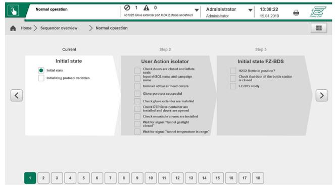
In case of a nonconformance, zenon triggers an alarm, then displays the required next steps on the user interface.
