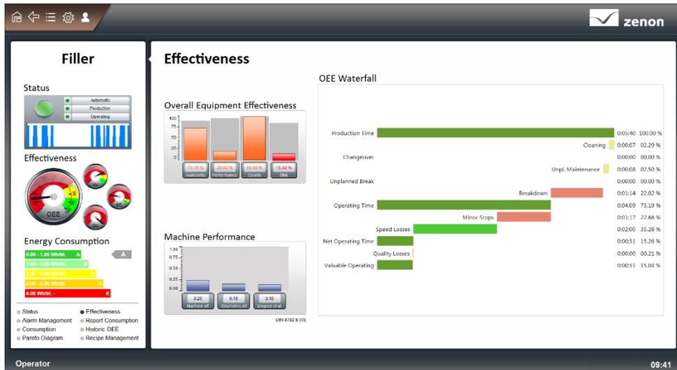
Figure 4: Analysis using an OEE Waterfall Diagram in zenon
