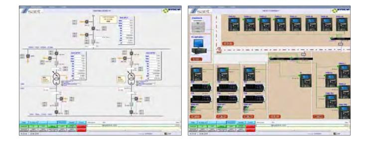
61850 protection relays, a SCADA system and a power quality recorder. SAET decided to entrust the substation system supervision tasks to the COPA-DATA zenon and straton software. The integration of the SCADA with the national grid is completed by way of the gateway with the ICE 60870-104 protocol integrated into zenon and by way of the events recording in COMTRADE format.
