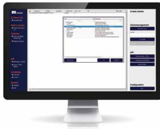
Figure: The context list allows manually-entered data to be arranged. So alarm causes, for example, can be pre-defined and thereby used for later analyses.
