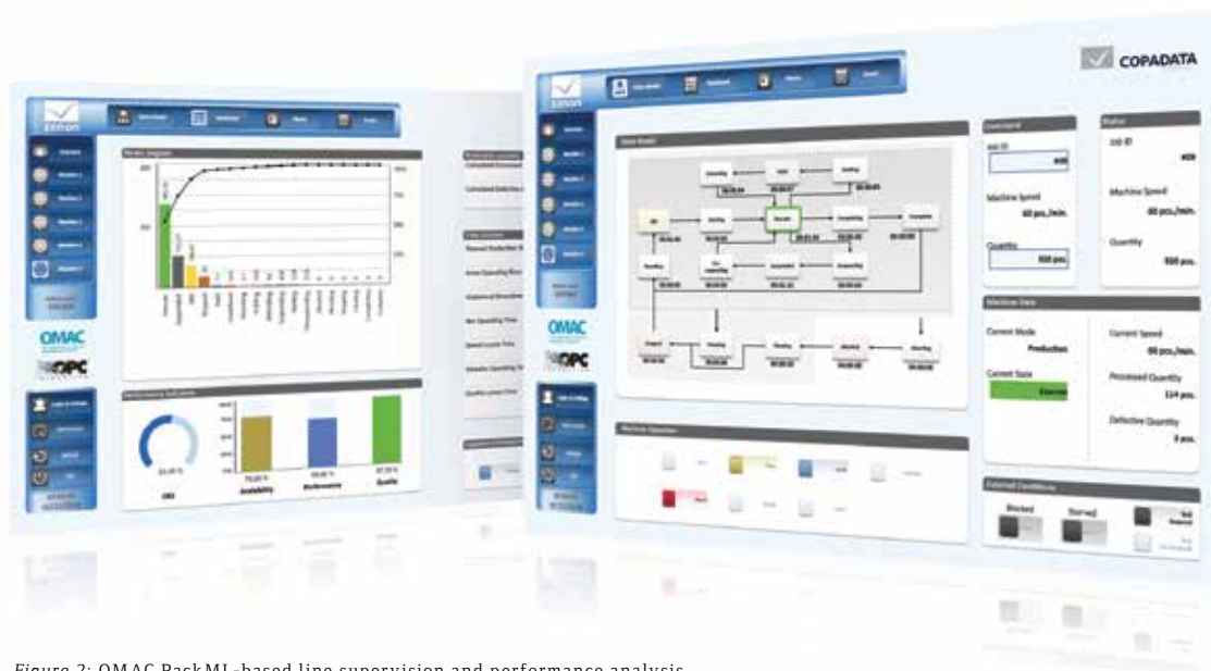
Figure 2: OMAC PackML-based line supervision and performance analysis.
