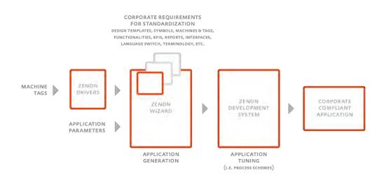
Figure 5: The flow of engineering information when using "Automatic Engineering".
