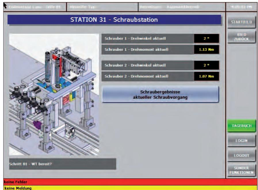
*zenon provides the user with all necessary information, such as the angle of rotation or torque, at a glance.*
