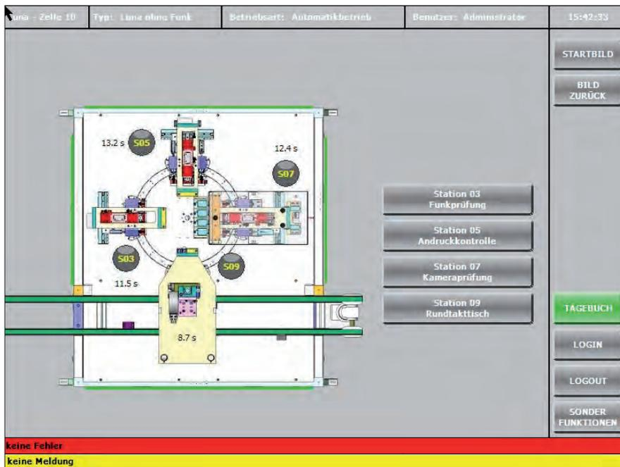
For a better overview, machine and equipment layouts are integrated into the application and the control panels at the individual stations.
