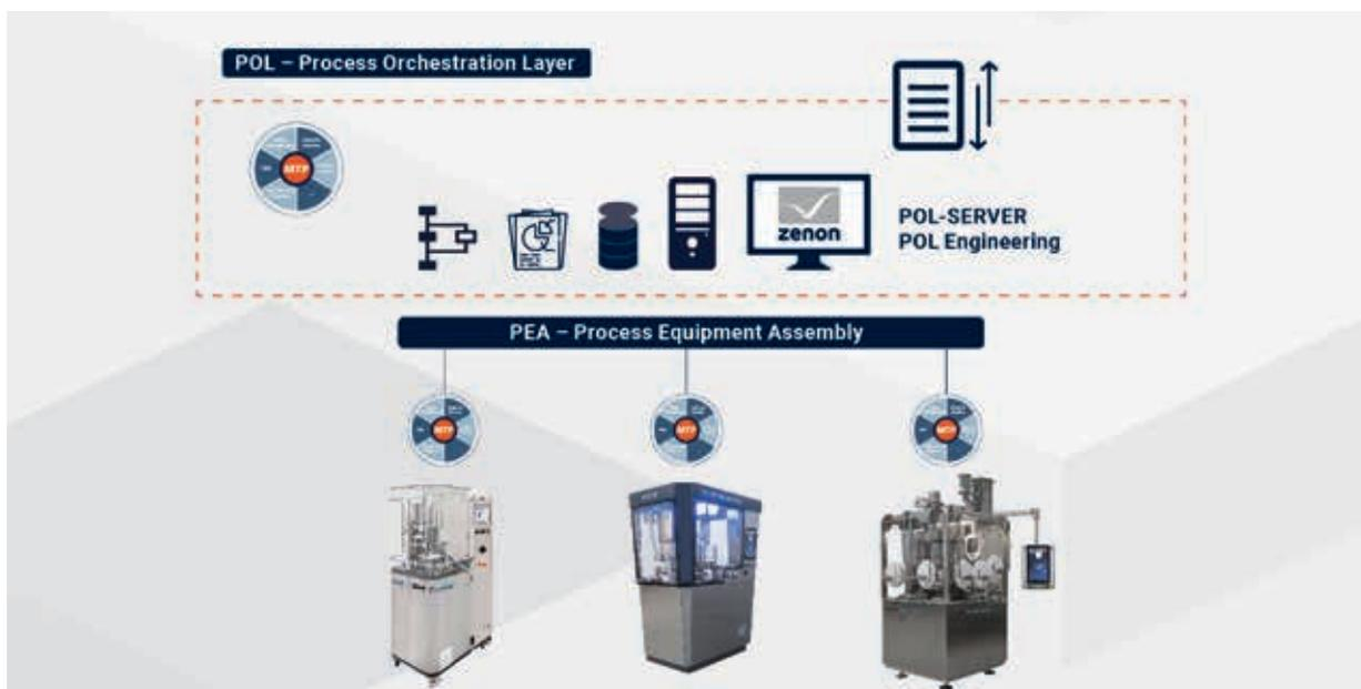
Figure 2: Integration of MG2 machines into POL via MTP.
