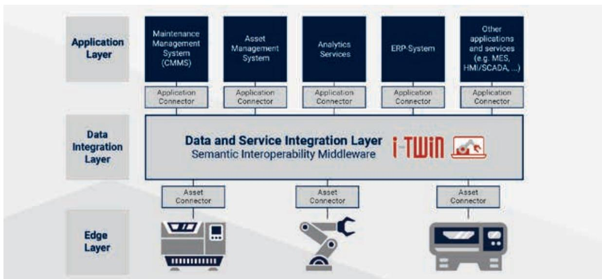
Figure 3: Industrial communication via the Data Integration Layer (i-Twin) – © Salzburg Research.
