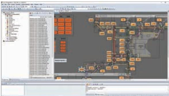
Budapest Airport’s control system department used the zenon software platform to create a high-level operating system for the air-ground lighting system including twelve redundant PLCs.
