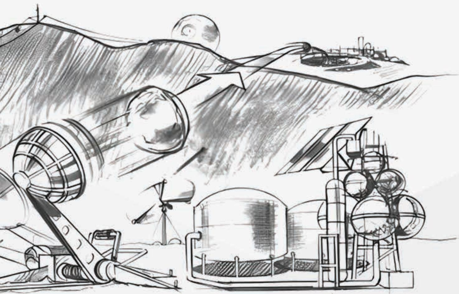
Multiple approaches for the extraction of oxygen from regolith (lunar soil) exist. For industrial scale deployments, some method is needed to transport the upper few meters of regolith, containing sharp, glass like particles, to the processing plant. With minimal equipment wear and low maintenance requirements, one approach for transport is based on ballistic conveying. Imagine a smarter factory like this!
