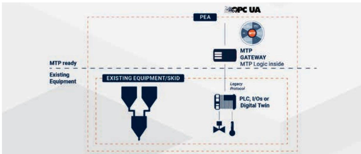
Figure 1: MTP Gateway for connecting existing equipment with MTP.
