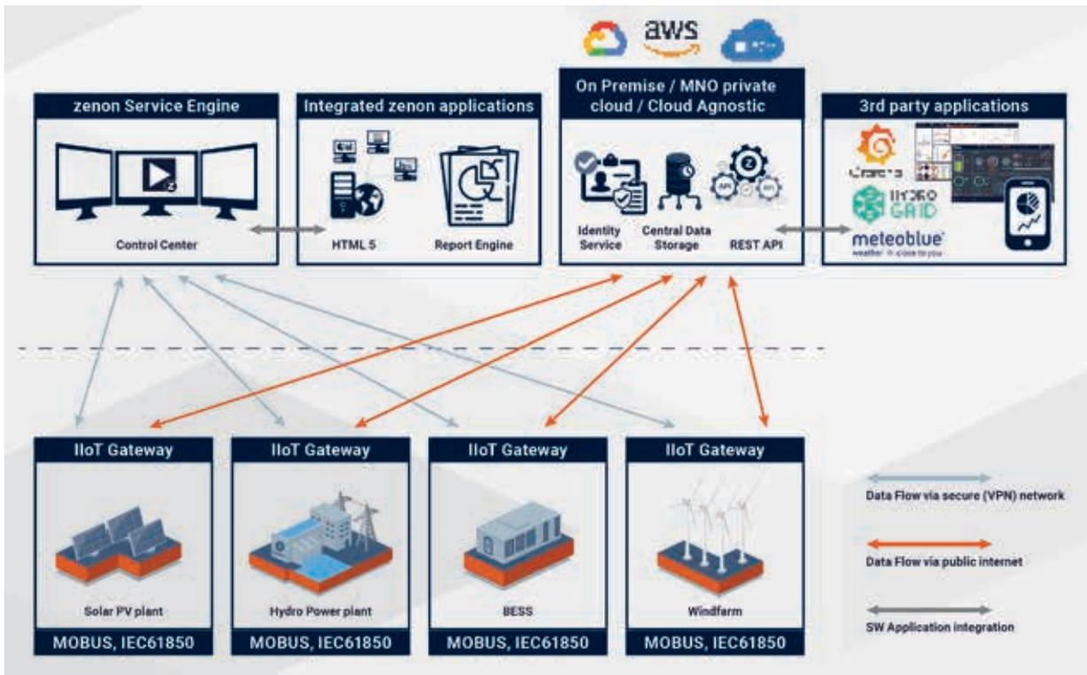
In addition, zenon IIoT Services includes a REST API service, enabling IT applications that need data from the asset to combine this information in dashboards, data analytics, and predictive maintenance applications. With zenon, O&M companies can offer a mobile-device application to site owners utilizing zenon IIoT Services, so that owners can see the sites are up and running at full efficiency and monitor how much energy and revenue they are generating.
