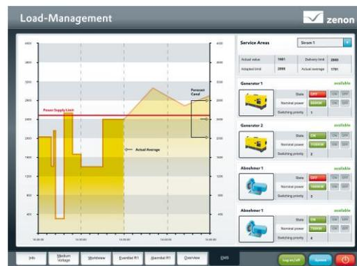
Figure 2: Avoiding expensive peak loads with zenon Load Management module.
