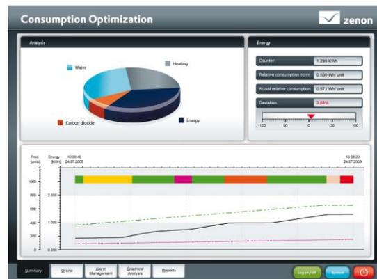
Figure 1: zenon calculates and presents the Energy Performance Indicators (EPIs) in real-time, in correlation with production information.
