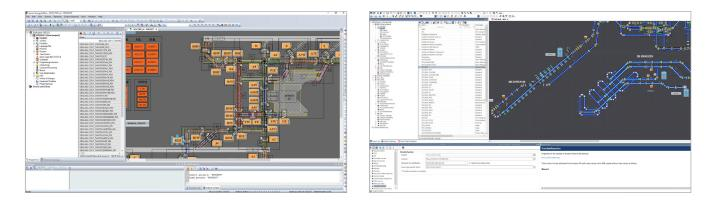
Budapest Airport's control system department used the zenon software platform to create a high-level operating system for the air-ground lighting system with its twelve redundant PLCs. The visualization for the baggage handling system with its more than 1,000 conveyors was created in two weeks purely by parameter setting.
