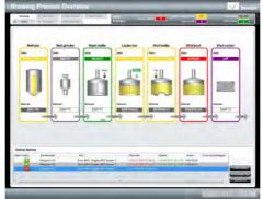
Figure 2: Beer brewing process visualization and control in zenon.
