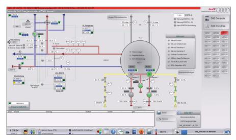
The car manufacturer's objective was to set up a central control room allowing the control and monitoring of energy and production materials for over 15 buildings, over a factory area of 395 hectares.
