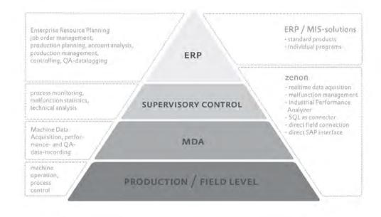
Automation software: zenon functions as a HMI and SCADA system from the machine through to the control room with interfaces to superordinate systems
