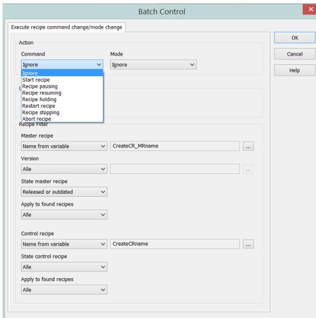
The figure above displays the 'execute recipe command' function to start and control an existing Control Recipe.
