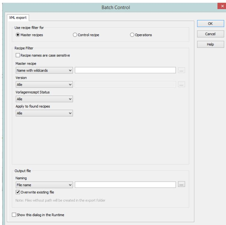
The function requires the specific Master Recipe name, together with version and status information if needed. The Master Recipe is exported to a static file location, or a location provided in a variable. Similar to the import function previously defined. This function can be specified and commanded by an external system such as a MES or ERP for example.
