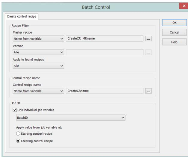
The above dialog provides an example function to create a new Control Recipe, with variables containing the Master and Control recipe name. In this example the Job ID is also requested, which is also contained in a specific variable. Therefore if this function call was to be used by a MES/ERP system, the call would require:
