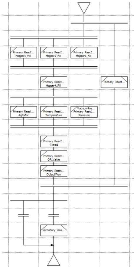
There is a second recipe editor in zenon. The Matrix editor uses the same structure with phases and operations separating the equipment control from the process control in the recipe.
