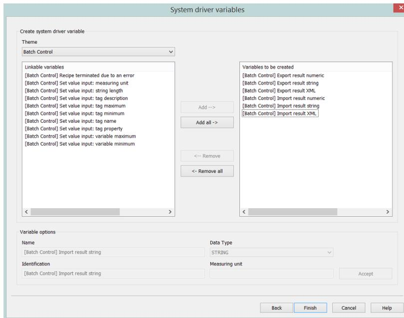
The two variables of interest are '[Batch Control] Export result numeric' and '[Batch Control] Import result numeric'. These provide a status on the recipe transfer, thus handling transitions and transfer errors, the help description is given below.
