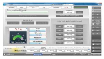
An up-to-date OEE overview is always available on the panel, which is access-protected via a RFID login, and online via web clients - without manual data collection.
