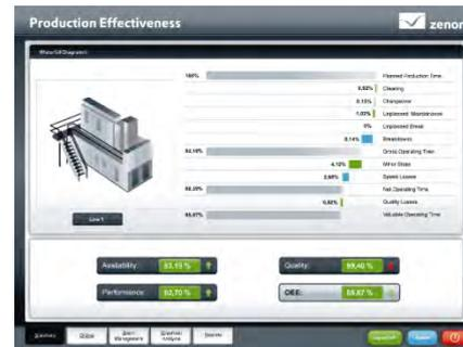
Figure 2: Analysis using an OEE Waterfall Diagram in zenon
