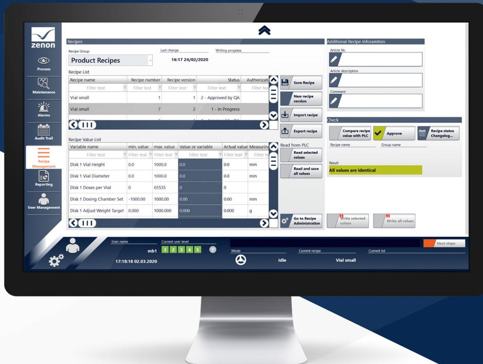
flow management, and recipe management are an integral part of the software platform. Engineering with zenon also provides versioning, change history and documentation to support the validation process. Detailed diagnostic options assist further; for example, to quickly identify problems in communication.
